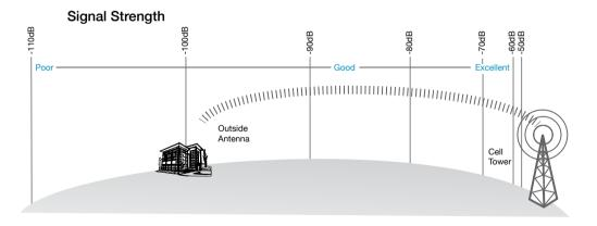
2. Select a location away from buildings, walls, trees, hills, and other terrain features that can block or reflect wireless signals (12-inch clear radius is recommended).
