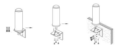
Note: If desired surface for installation plate is wood or concrete, wood or masonry screws for L-plate will have to be purchased separately.
