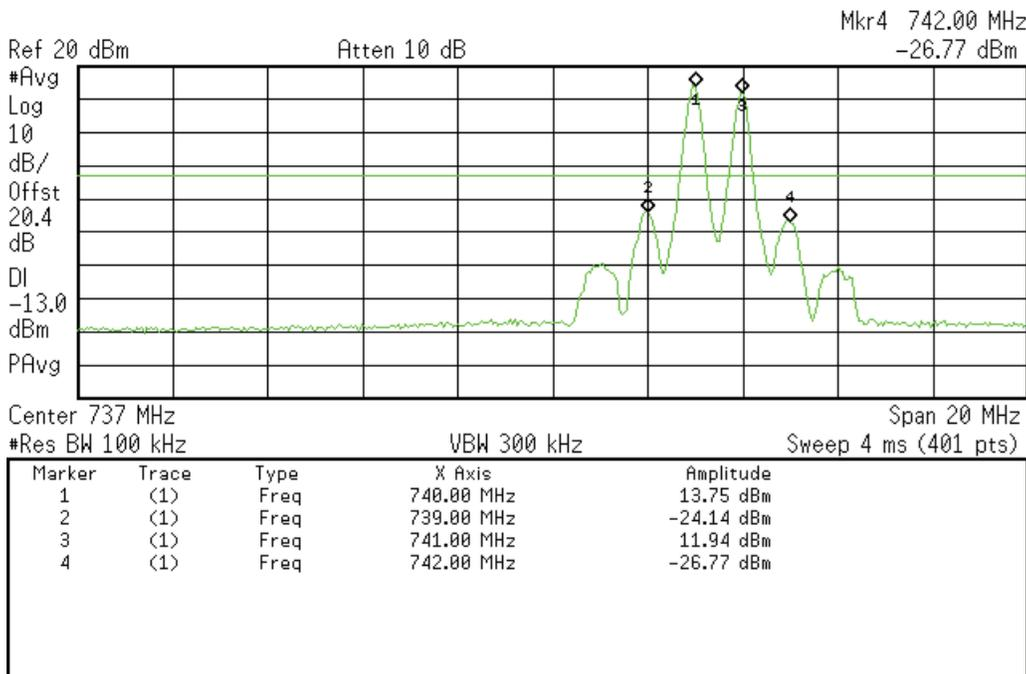
**Intermodulation Downlink Test Results at 6db above AGC (GSM Signal)
