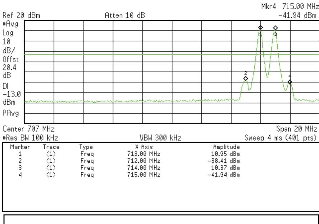
**Intermodulation Uplink Test Results at 3db above AGC (GSM Signal)
