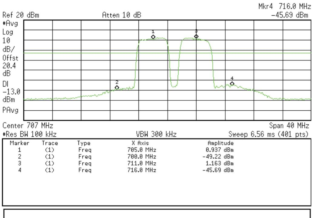
**Intermodulation Uplink Test Results at 6db above AGC (CDMA Signal)
