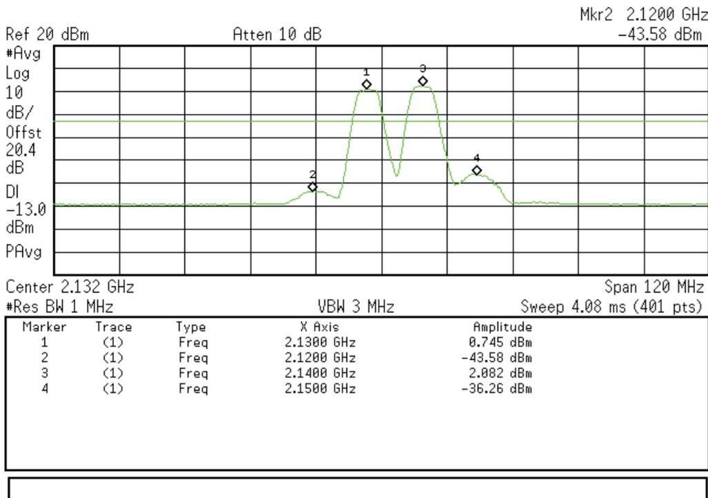
**Intermodulation Downlink Test Results at 3db above AGC (CDMA Signal)
