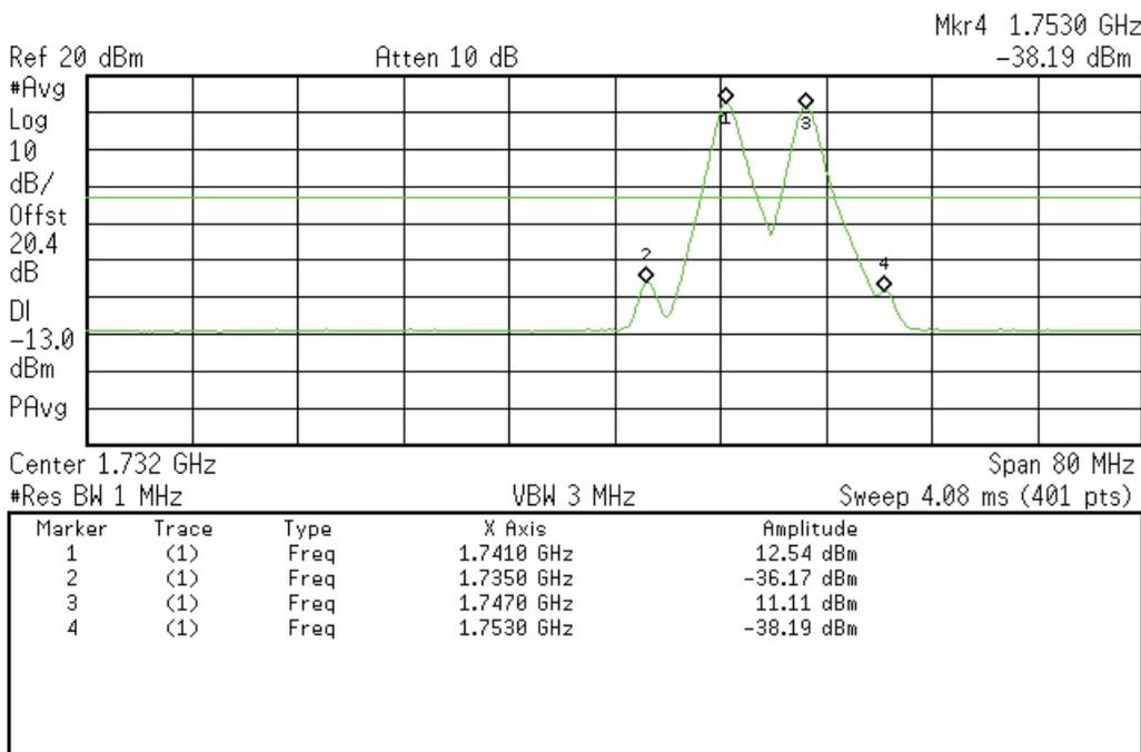
**Intermodulation Uplink Test Results at 6db above AGC (GSM Signal)
