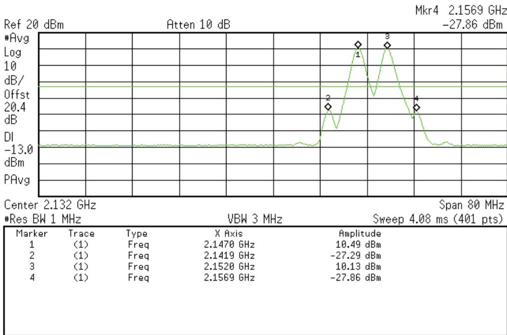
**Intermodulation Downlink Test Results at AGC (CDMA Signal)
