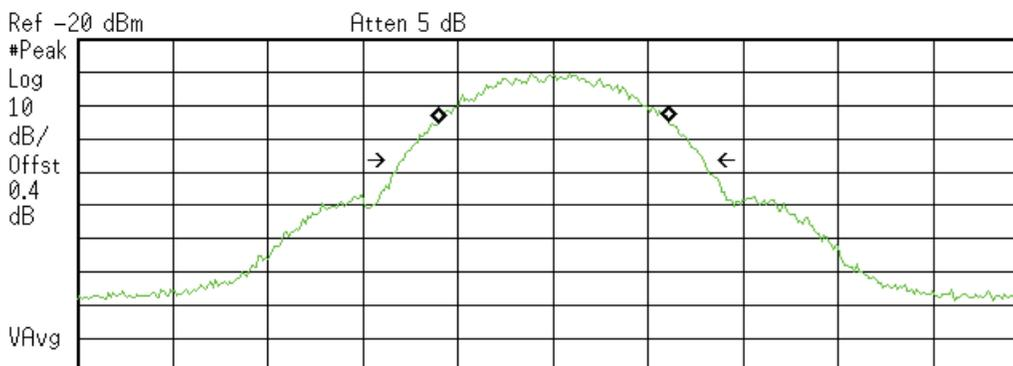
Center 1.732 GHz Span 1 MHz
