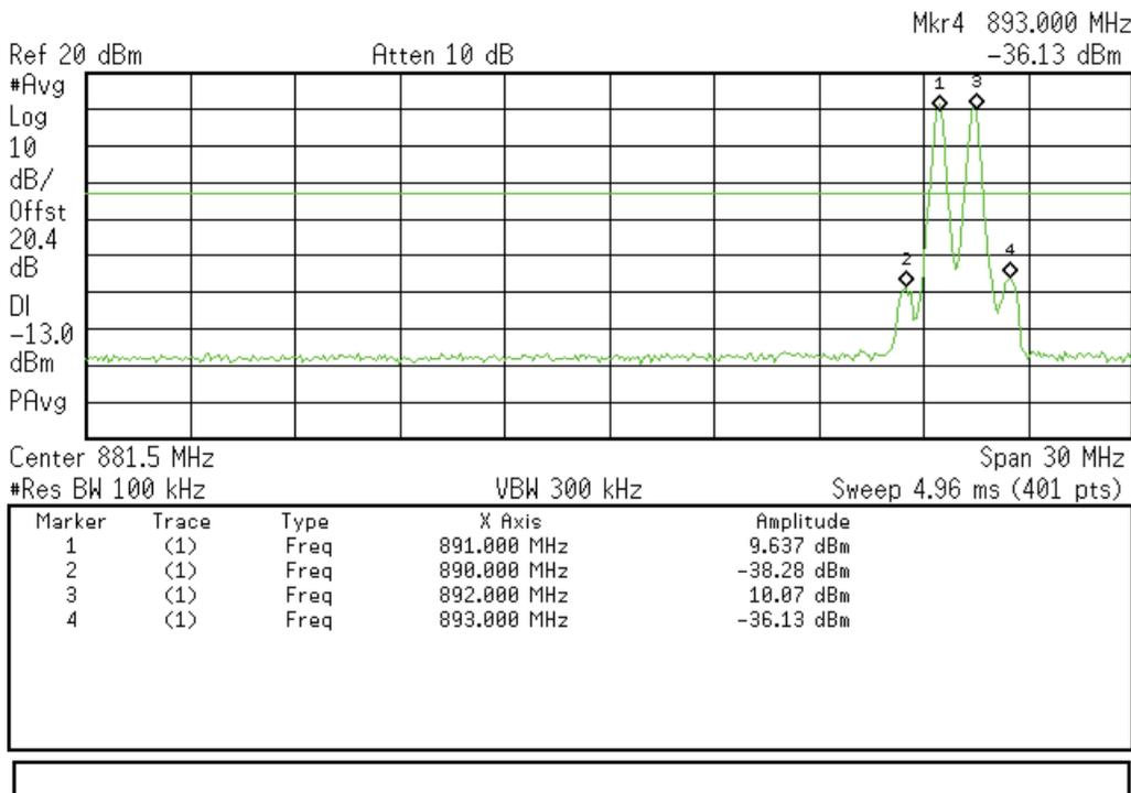
**Intermodulation Downlink Test Results at 6db above AGC (GSM Signal)
