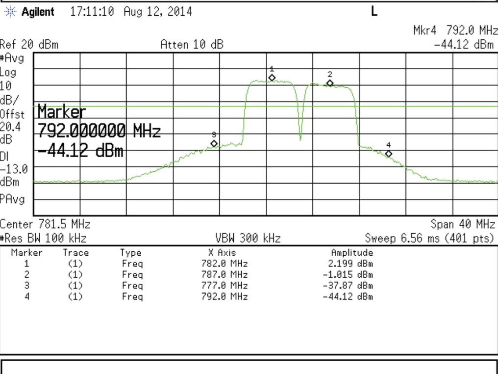
**Intermodulation Uplink Test Results at AGC (CDMA Signal)
