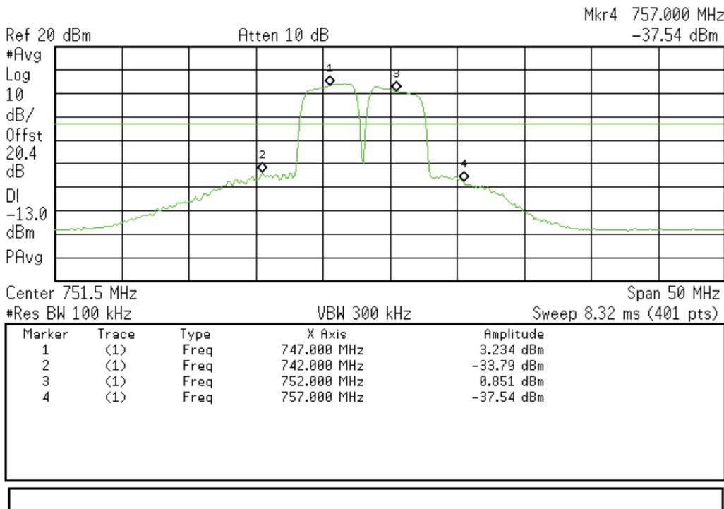
**Intermodulation Downlink Test Results at AGC (CDMA Signal)
