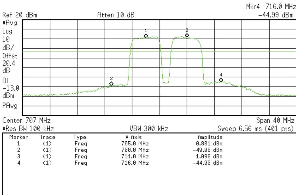
**Intermodulation Uplink Test Results at AGC (CDMA Signal)
