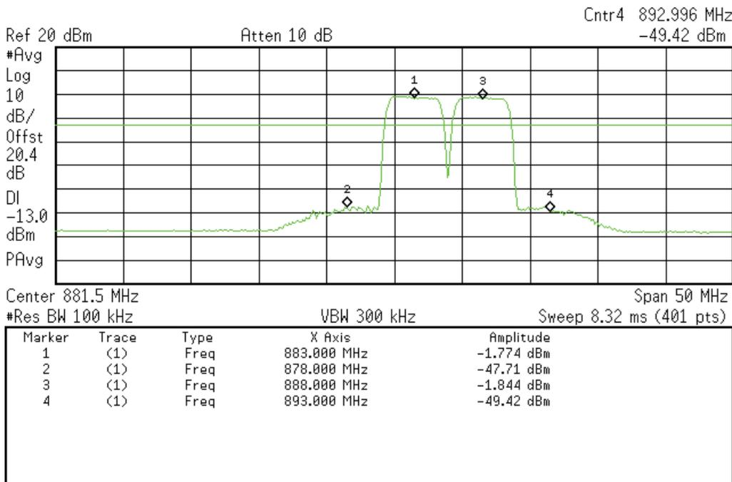
**Intermodulation Downlink Test Results at 6db above AGC (CDMA Signal)
