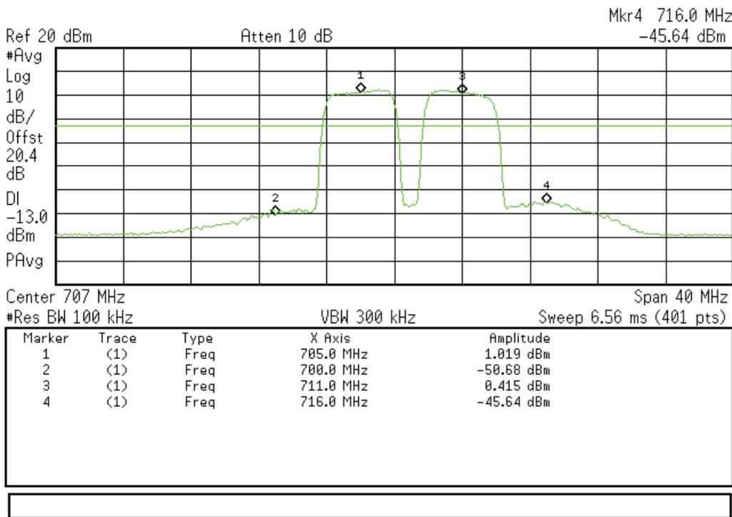
**Intermodulation Uplink Test Results at 3db above AGC (CDMA Signal)
