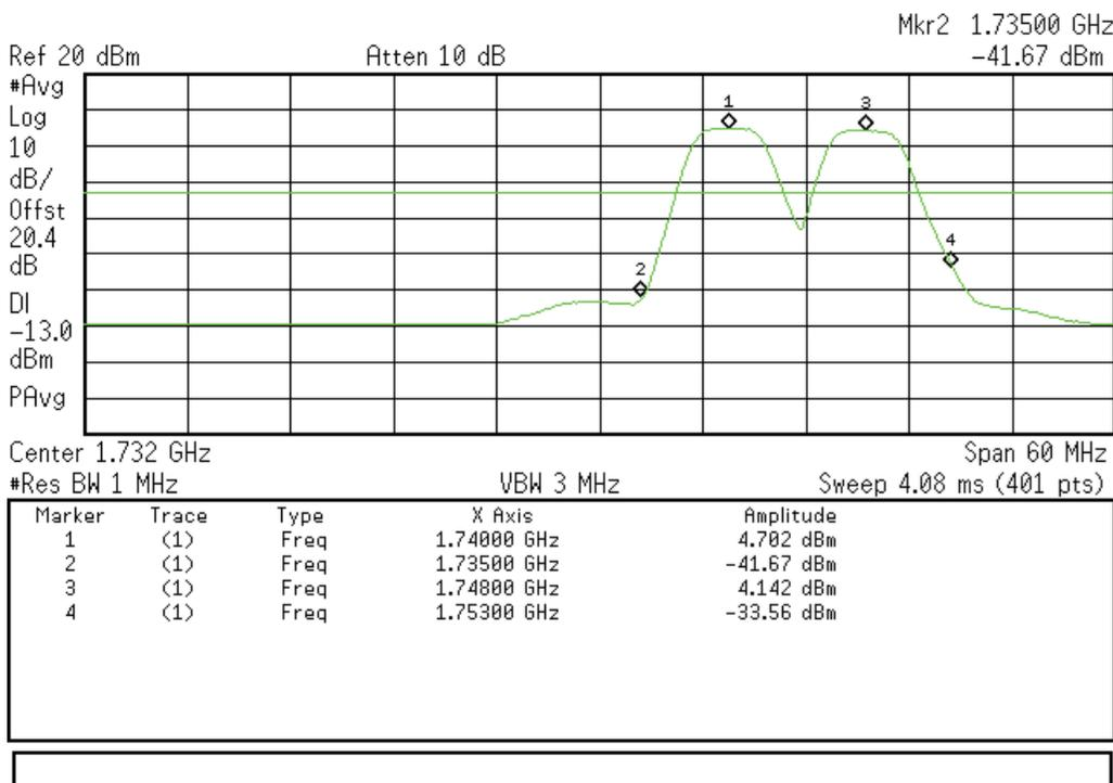
**Intermodulation Uplink Test Results at AGC (CDMA Signal)
