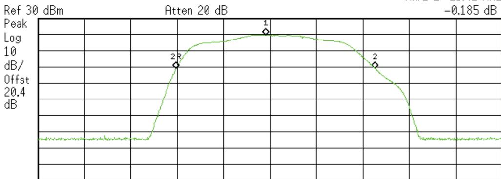
Center 781.5 MHz Span 50 MHz
