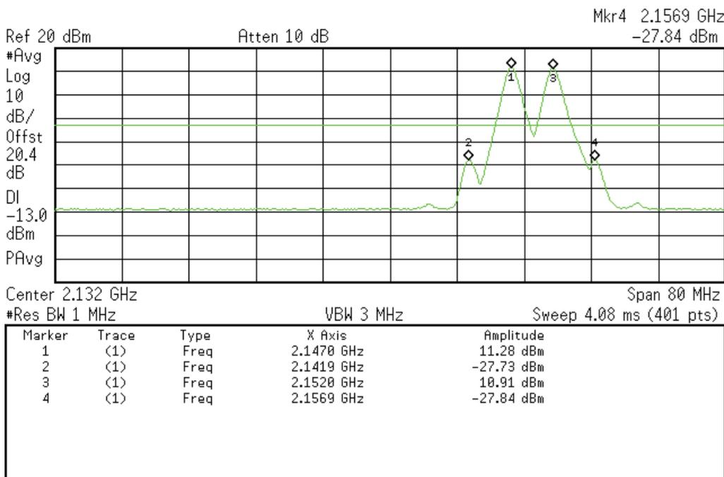
**Intermodulation Downlink Test Results at 3db above AGC (GSM Signal)
