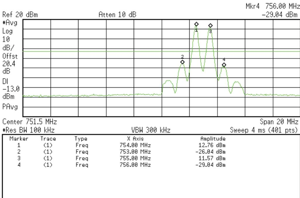
**Intermodulation Downlink Test Results at AGC (GSM Signal)
