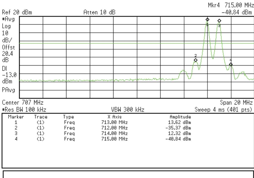
Intermodulation Uplink Test Results at 6db above AGC (GSM Signal)
