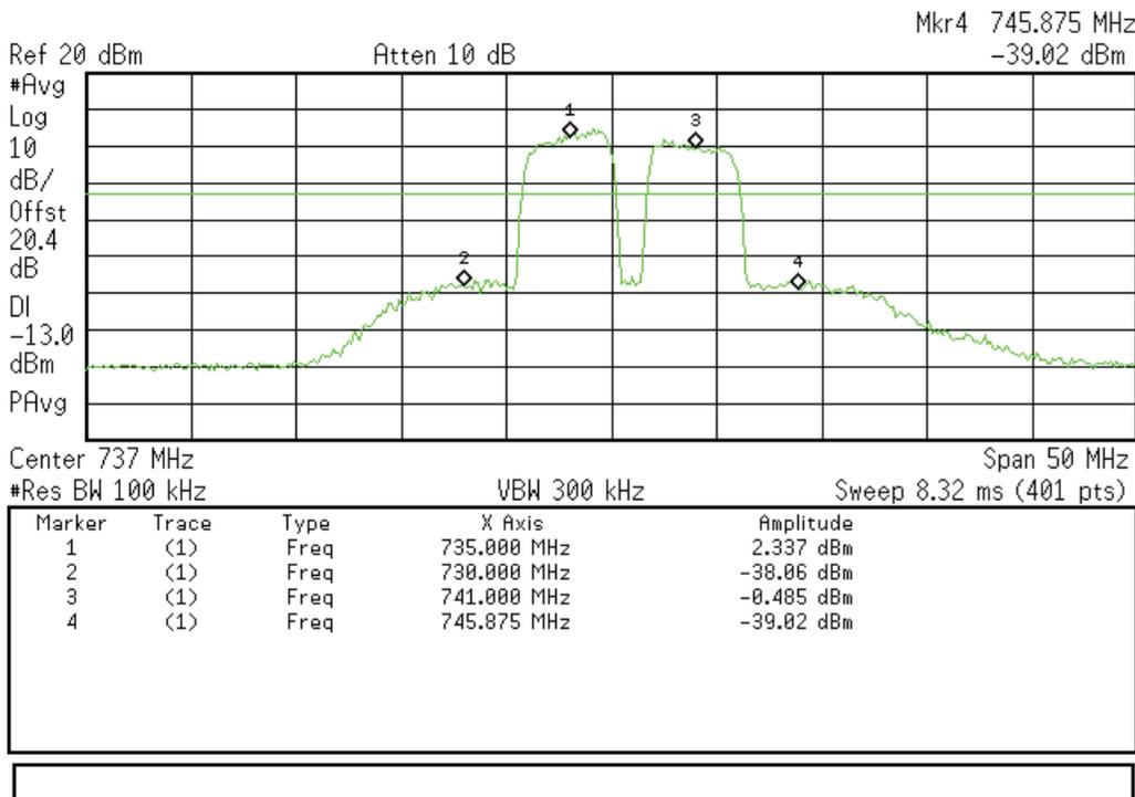
**Intermodulation Downlink Test Results at 6db above AGC (CDMA Signal)
