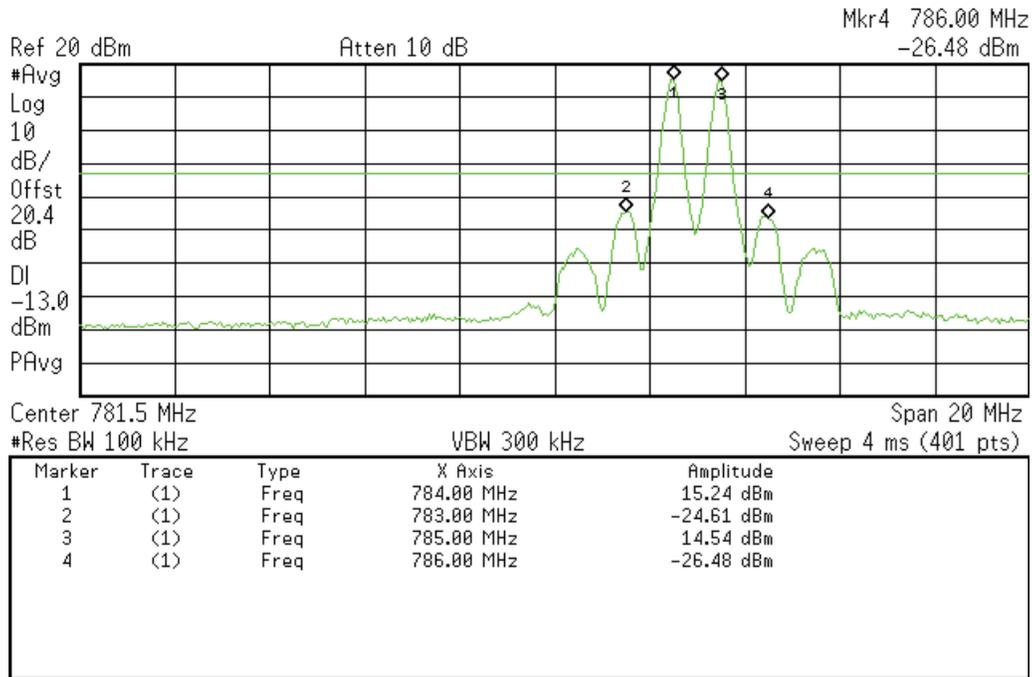
**Intermodulation Uplink Test Results at AGC (GSM Signal)
