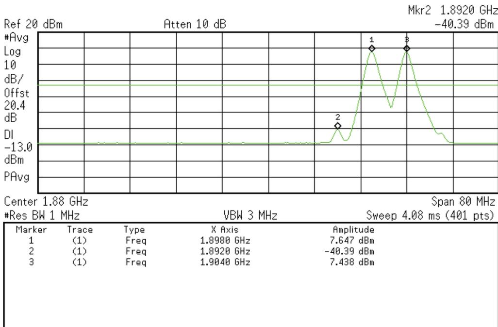
**Intermodulation Uplink Test Results at 3db above AGC (GSM Signal)
