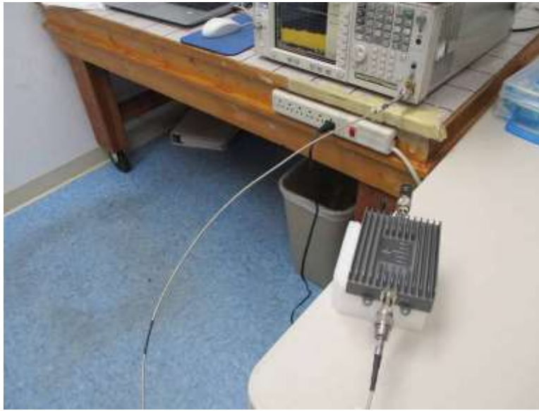
Section 7.7 Max Noise Test Setup
