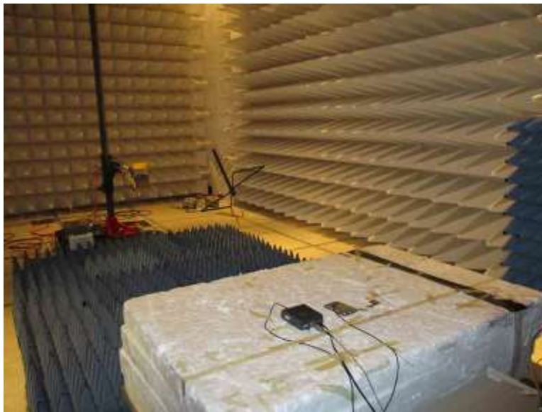
Section 7.12, Above 1GHz Cone placement Test Setup
