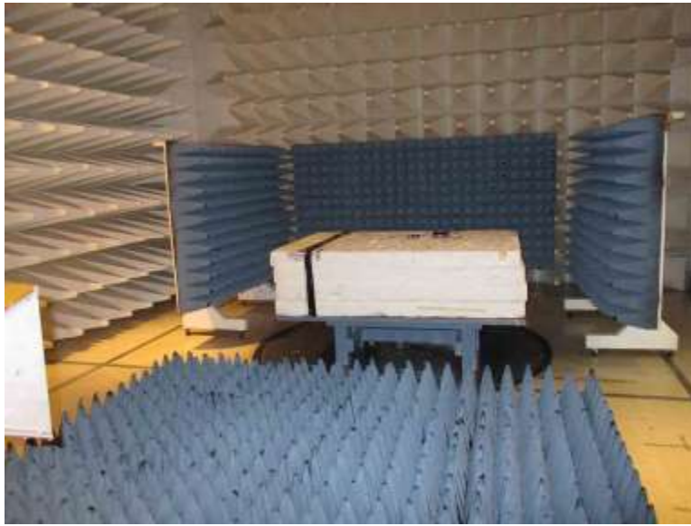
Section 7.12, Above 1GHz Cone placement Test Setup
