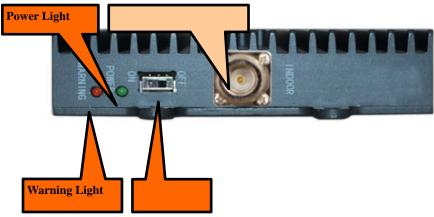
STEP 6. Turn the Power Switch on
