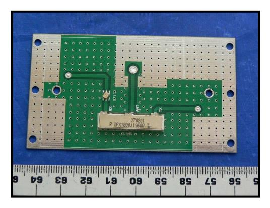
**1.8 RF input board solder side view for downlink**
