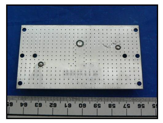
1.9 RF input board component side view for uplink
