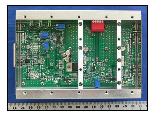
**1.3** Downlink board Component side View
