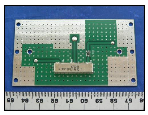
1.10 RF input board solder side view for uplink
