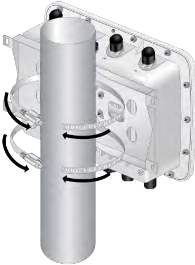
Figure 35. Wrapping the Pole Straps Around the Pole
