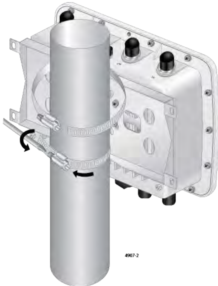
Figure 37. Tightening the Straps
