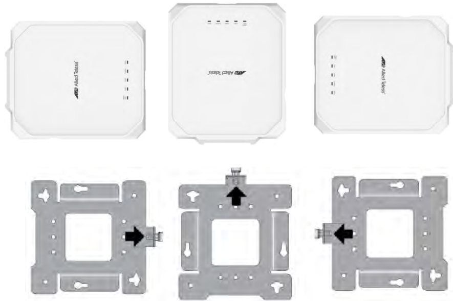
Figure 27. Seating the Access Point on the Mounting Bracket
