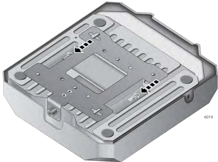
Figure 14. Attaching the Mounting Bracket on the Access Point
