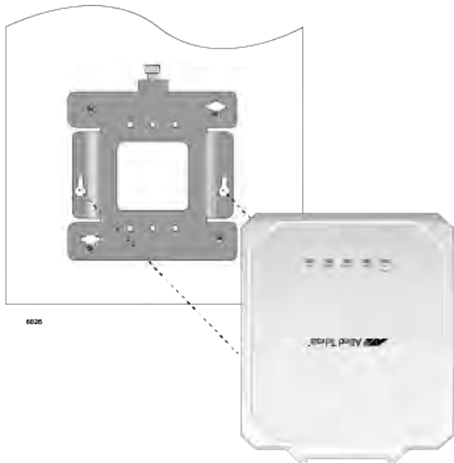
Figure 26. Installing the Access Point on the Mounting Bracket
