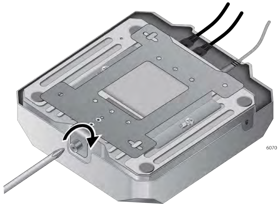
Figure 27. Tightening the Mounting Bracket Thumbscrew
