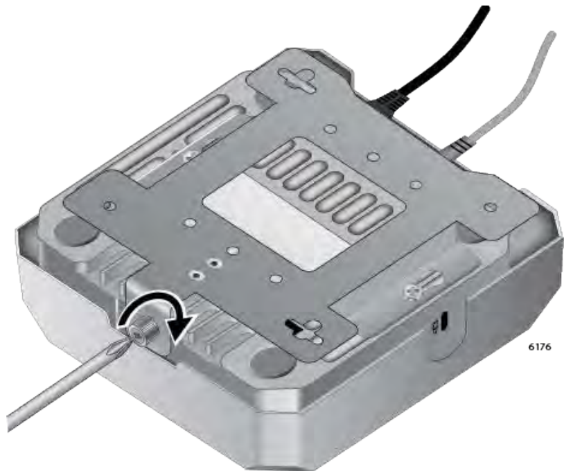
Figure 22. Tightening the Mounting Bracket Thumbscrew
