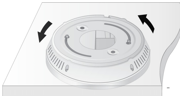
Figure 26. Turning the Access Point to Secure to the Mounting Base
