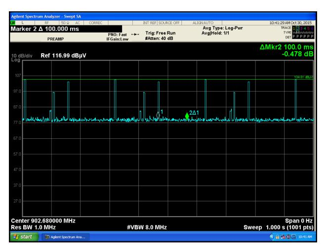
$\begin{aligned} \text{Maximum Pulses in any 100 ms period} &= 1 \\ \text{Duty Cycle} &= 4.000 \text{ percent} \end{aligned}$  The maximum 20 dB Peak to Average ratio can be used
