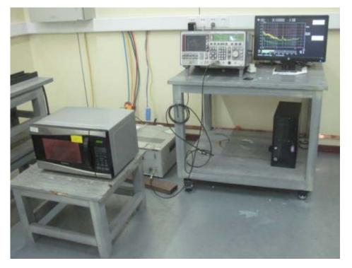
Radiated Emission Test Set-up (30 -1,000MHz):
