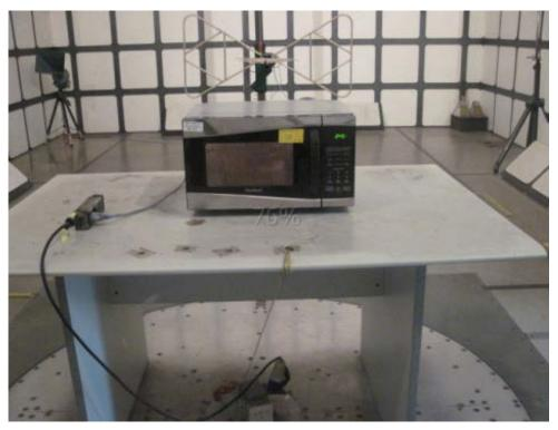
Radiated Emission Test Set-up (1-25GHz):
