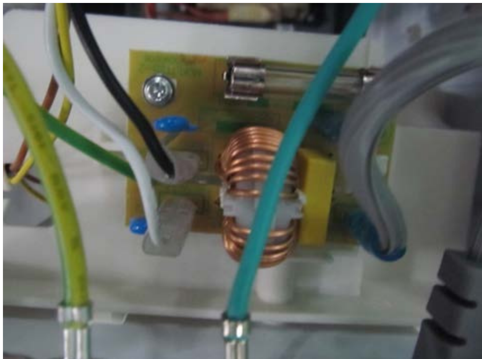
Power Filter Board Top View
