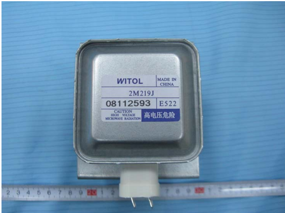
EUT – Magnetron View
