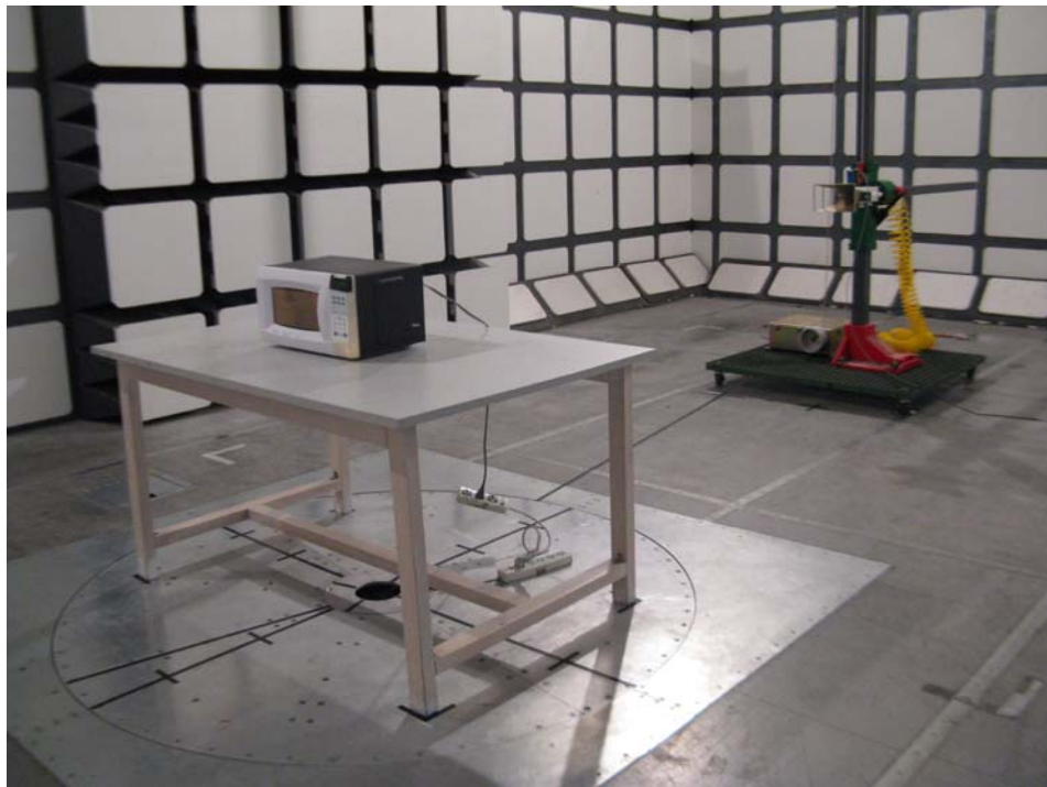
Radiated Emissions - Rear View (Above 1 GHz)
