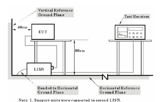
The setup of EUT is according with per MP-5: 1986 measurement procedure. Specification used was with the FCC Part 18.
