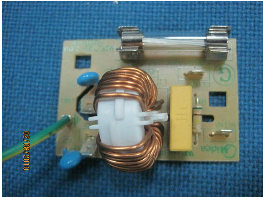
Power Filter Board Top View
