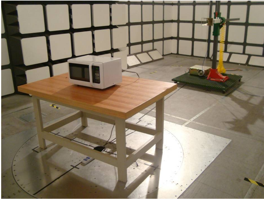
Radiated Emissions - Rear View (Above 1 GHz)
