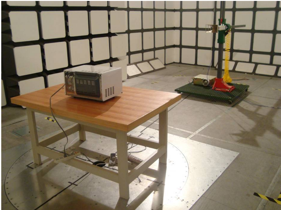
Radiated Emissions - Rear View (Above 1 GHz)
