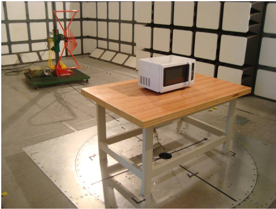
Radiated Emissions - Rear View (Below 1 GHz)
