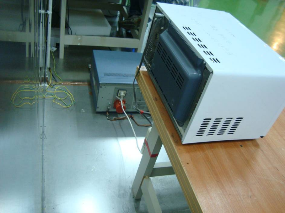
Conduction Emissions - Side View
