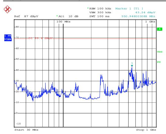
MD Microwave oven M/N:MM720ASF radiation emission Vertical
