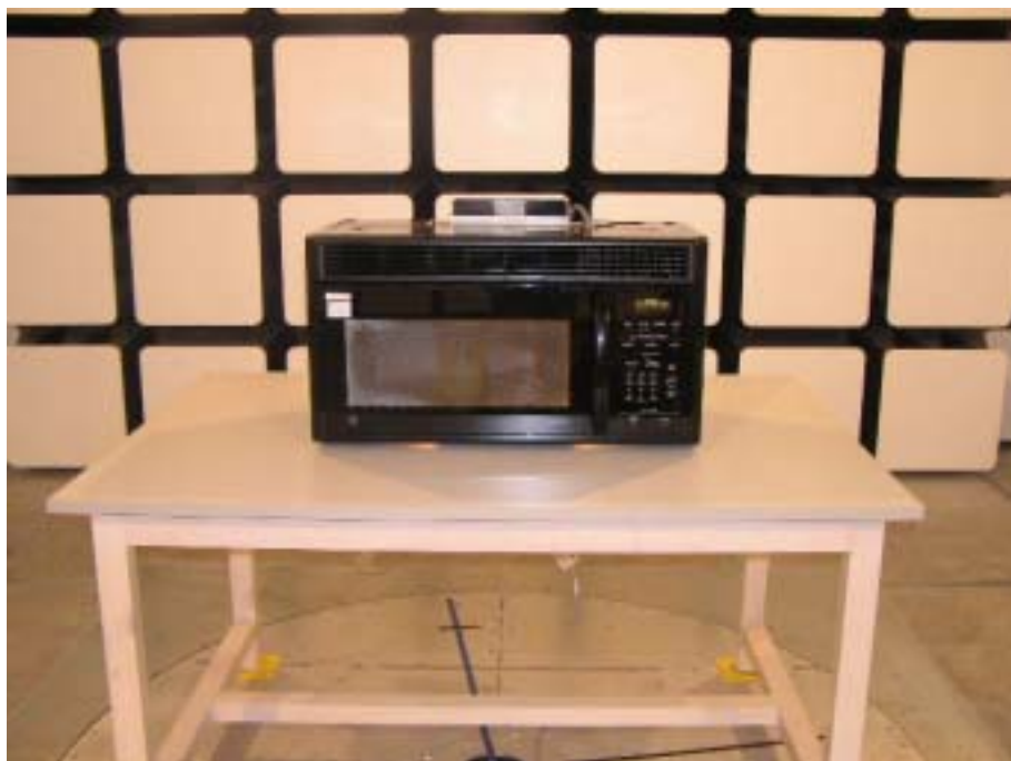
30MHz to 1000MHz:Radiated Emission - Rear View
