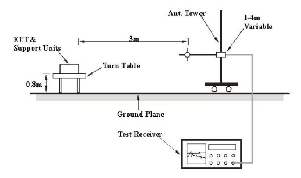
The radiated emission tests were performed in the 3 meters chamber B, using the setup accordance with the FCC MP - 5. The specification used was the FCC part 18 limits.
