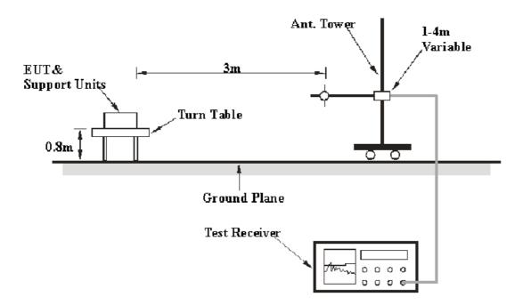
The radiated emission tests were performed in the 3 meters chamber A test site, using the setup accordance with the FCC MP - 5. The specification used was the FCC part 18.
