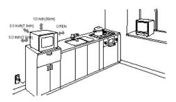
A minimum clearance of 3.0 inch (7.5cm) is required between the oven and any adjacent wall.One side must be open. on the cabinet surface.
