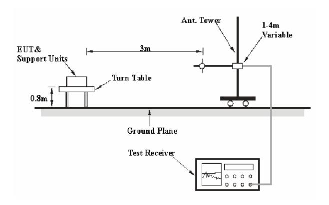
The radiated emission tests were performed in the 3 meters chamber A test site, using the setup accordance with the FCC MP - 5. The specification used was the FCC part 18 limits.
