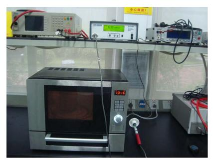
**Input Power Test Set-Up :**
