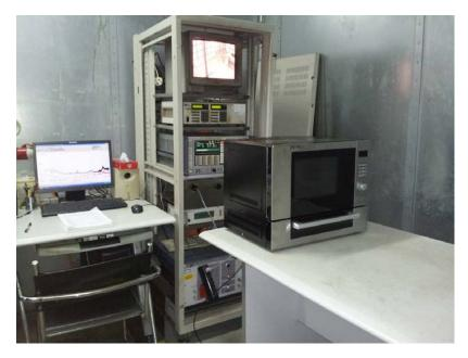
Radiated Emission Test Set-up (30 -1,000MHz):
