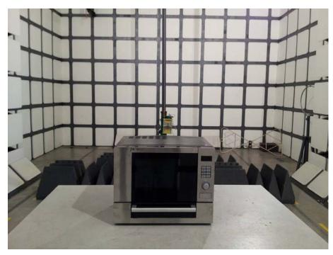
Radiated Emission Test Set-up (1-25GHz):
