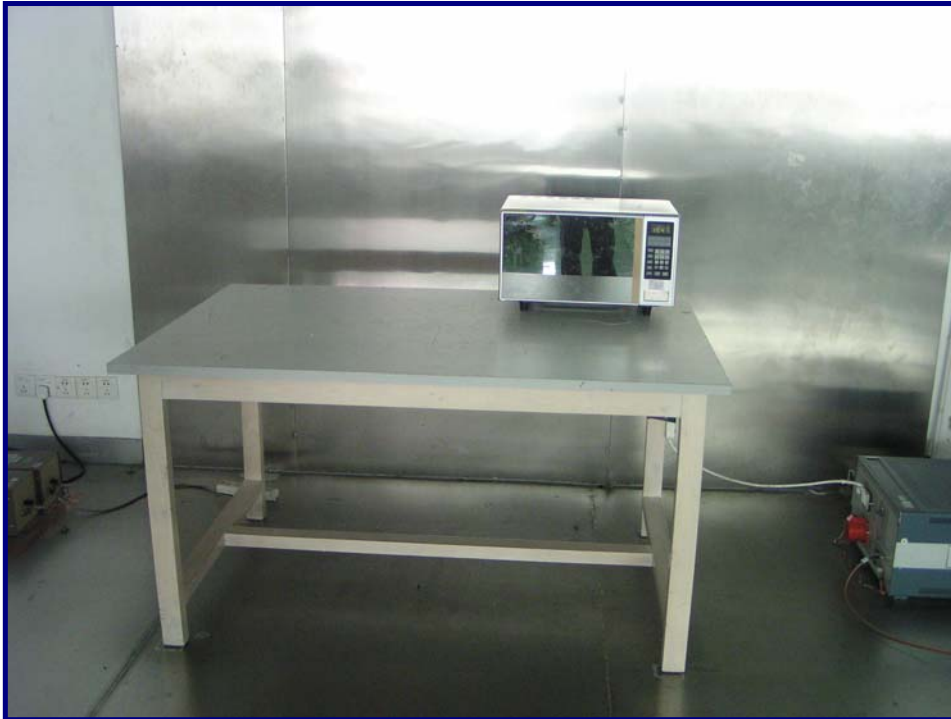
Conducted Emission - Front View
