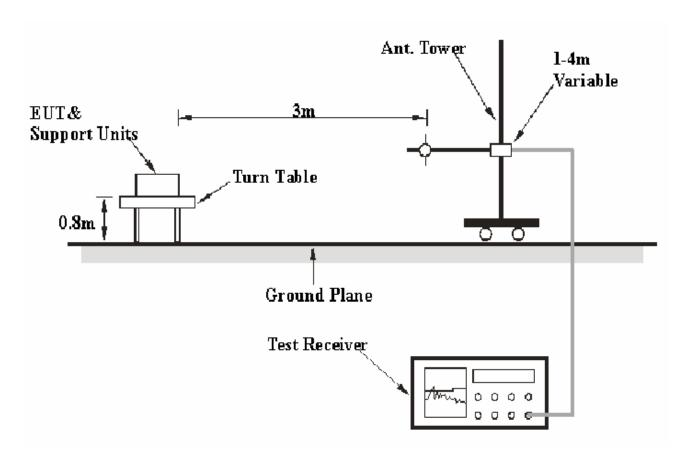
The radiated emission tests were performed in the 3 meters chamber B test site, using the setup accordance with the FCC MP - 5. The specification used was the FCC part 18 limits.
