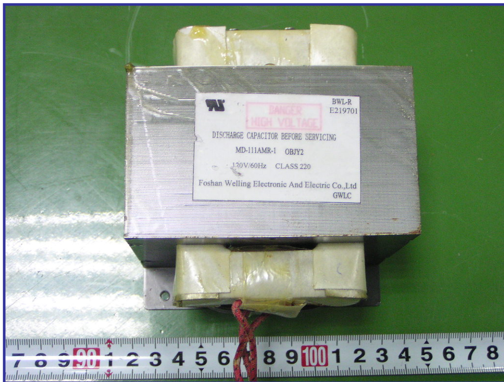
EUT -Transformer View
