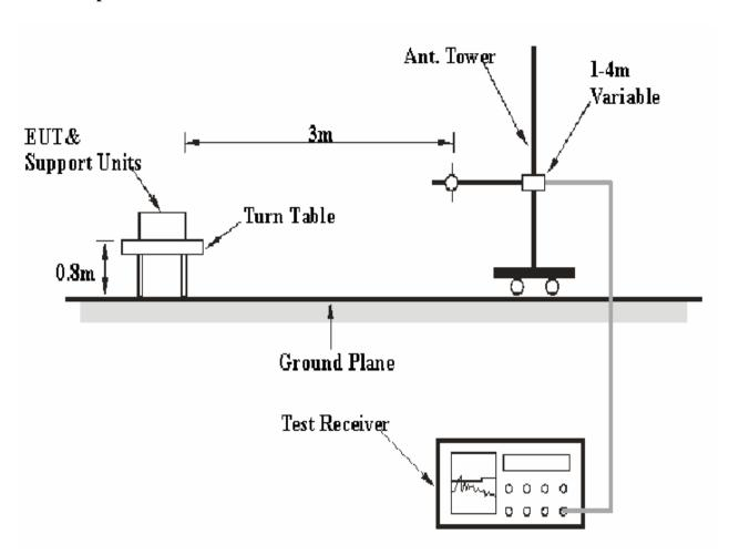
The radiated emission tests were performed in the 3 meters chamber A test site, using the setup accordance with the FCC MP - 5. The specification used was the FCC part 18 limits.
