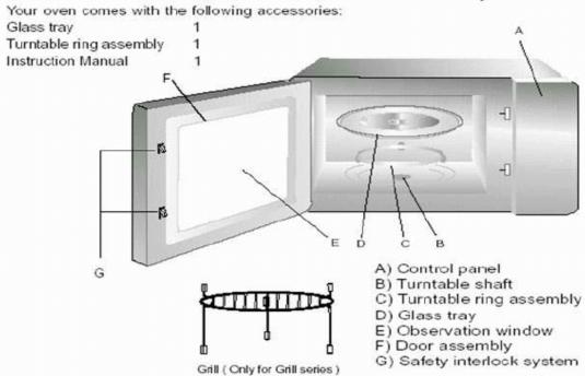
Shut off oven power if the door is opened during operation.
