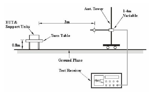
The radiated emission tests were performed in the 3 meters chamber B test site, using the setup accordance with the FCC MP - 5. The specification used was the FCC part 18 limits.
