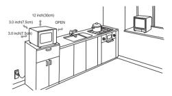
A minimum clearance of 3.0 inch (7.5cm) is required between the oven and any adjacent wall.One side must be open. on the cabinet surface.
