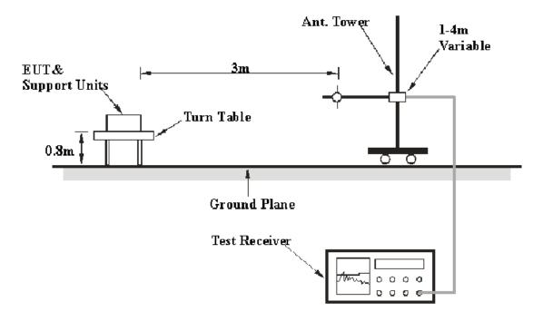
The radiated emission tests were performed in the open area 3-meter test site, using the setup accordance with the FCC MP - 5. The specification used was the FCC part 18 Subpart C limits.
