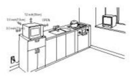
A minimum clearance of 3.0 inch (7.5cm) is required between the oven and any adjacent wall. One side must be open. on the cabinet surface.
