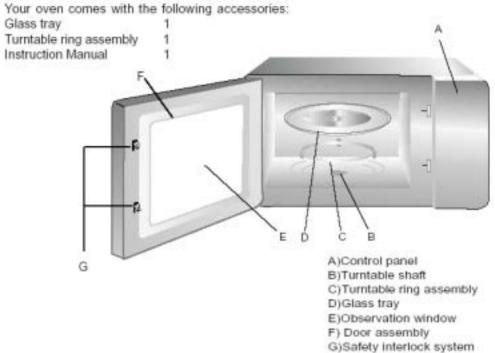
Shuts off oven power if door is opened during operation.
