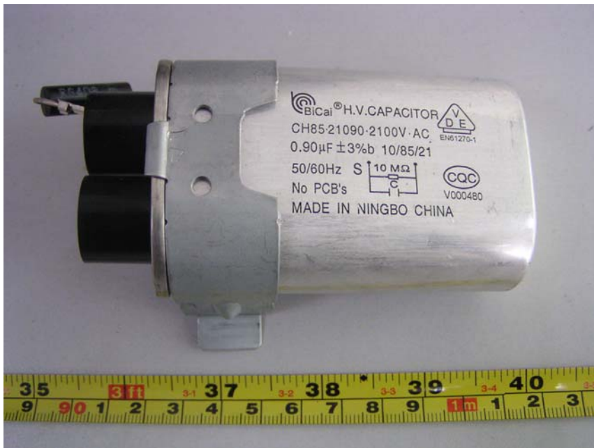
EUT -HV cap. View (1)
