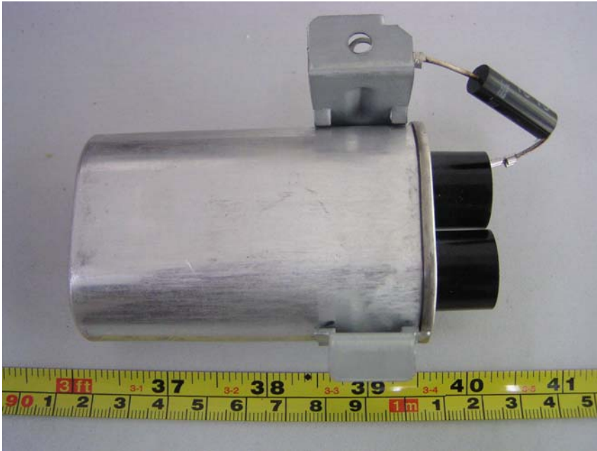
EUT -HV cap. View (2)
