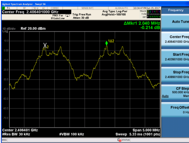
Channel Separation plot on channel 17-18
