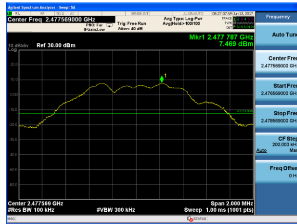
GFSK on channel 36
