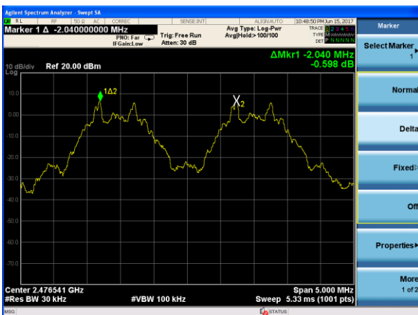
Channel Separation plot on channel 35-36
