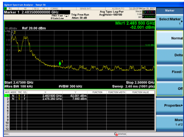
GFSK: Band Edge-High Channel (Hopping Mode)
