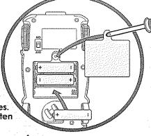
To Replace REMOTE CONTROL Batteries
