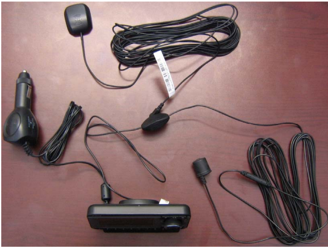
Antenna, Power Input, and Sure Connect External Setup
