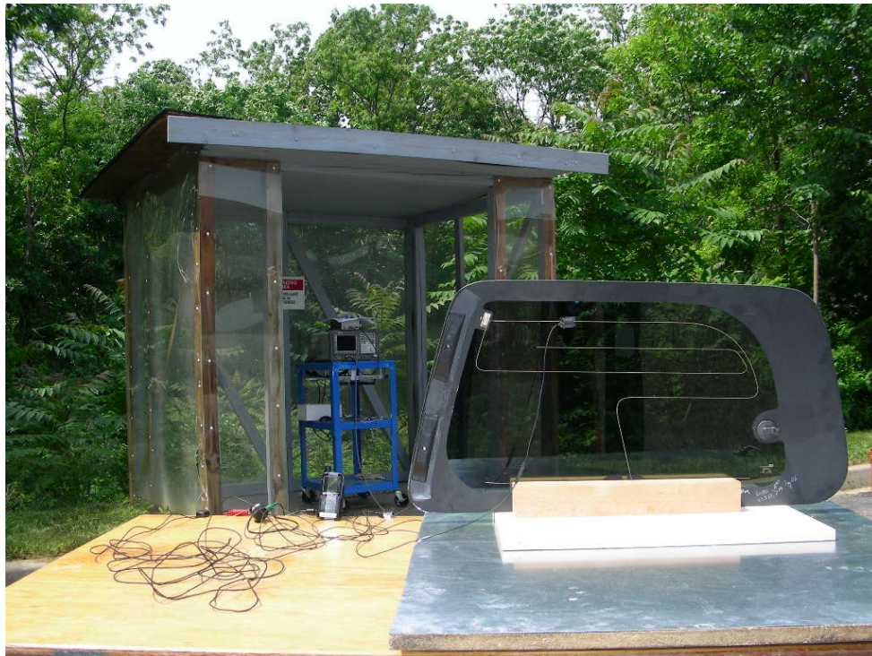
Figure 1-4. SureConnect with Glass Antenna Set-up – Test Configuration #7
