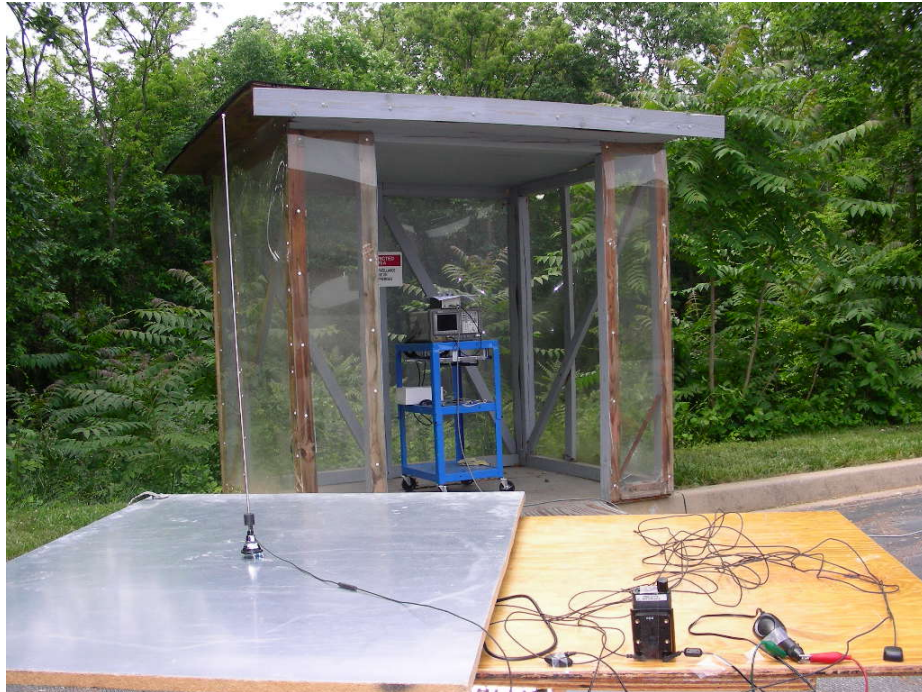
Figure 1-1. SureConnect with FM Antenna Set-up – Test Configuration #5
