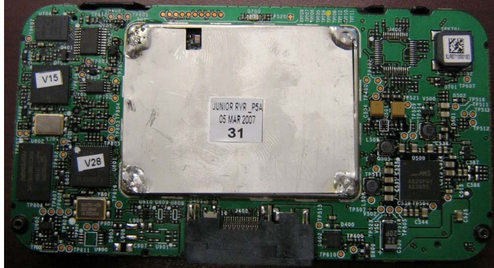
Back of PCB with shield
