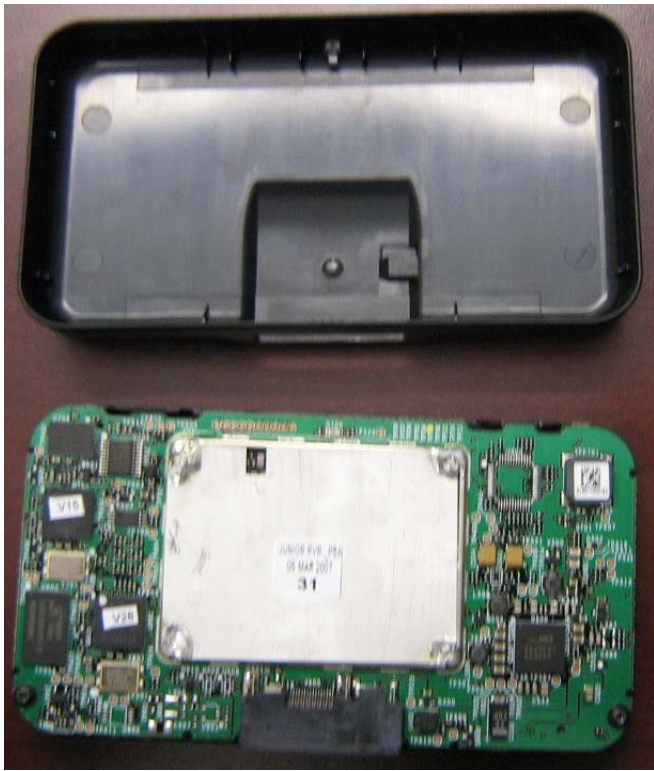
Case Open with PCB Inside
