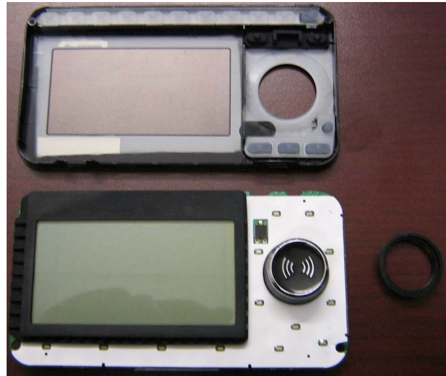
Case Open with PCBs Removed
