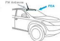
FRONT ROOF TOP MOUNTED FM ANTENNA
