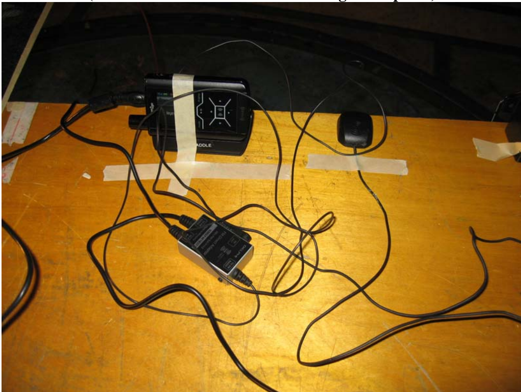
Photo 10 : Car Cradle using FM Direct Adapter (and FM aerial antenna attached to ground plane)
