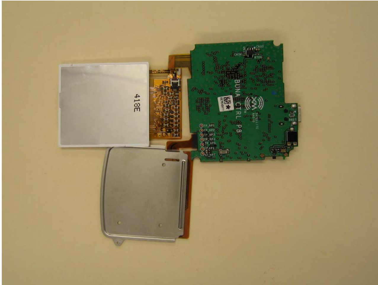
Controller Board - Back
