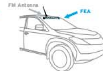
FRONT ROOF TOP MOUNTED FM ANTENNA
