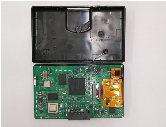
PCBA Rear View (w/back housing removed) PCBA Rear View (w/front housing & screws)
