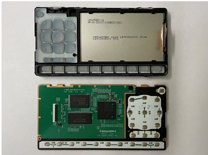
Front View with Front Housing, Keypad(s) and Display Removed
