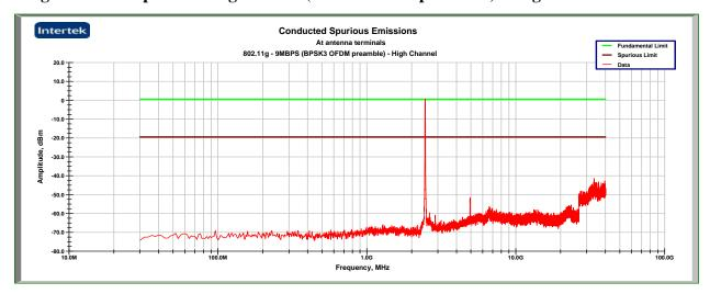
Lynx B1-802.11g - 9MPS (BPSK OFDM preamble) - High Channel
