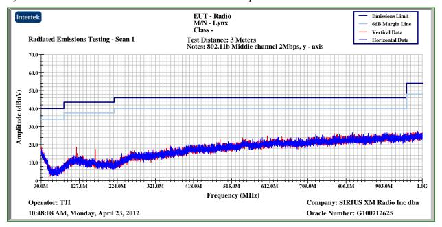
Lynx B - Peak Plot – 30MHz-1000MHz – 802.11b – 2.0Mbps – Middle Channel
