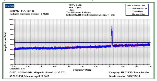
Lynx B - Peak Plot – 1000MHz-3000MHz – 802.11b – 2.0Mbps – Middle Channel
