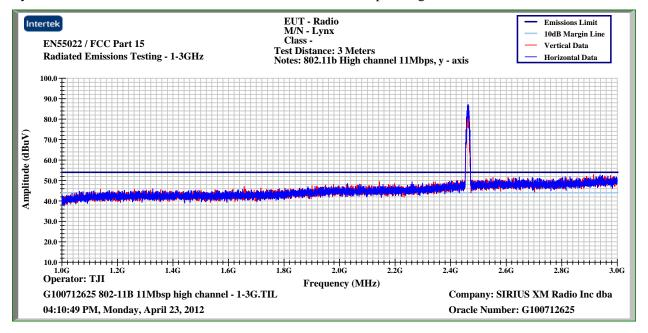
Lynx B - Peak Plot - 1000MHz-3000MHz - 802.11b - 11Mbps - High Channel
