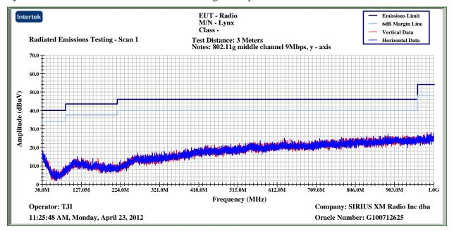
Lynx B - Peak Plot – 30MHz-1000MHz – 802.11g – 9Mbps – Middle Channel
