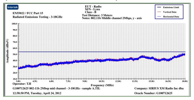
Lynx B - Peak Plot – 3000MHz-18000MHz – 802.11b – 2.0Mbps – Middle Channel
