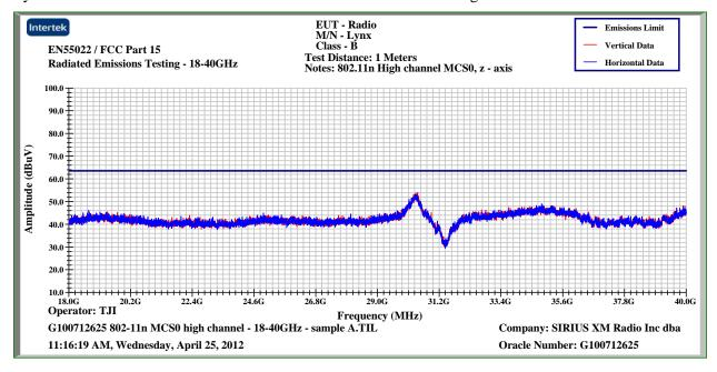
Lynx B - Peak Plot - 18000MHz-40000MHz - 802.11n - MCS0 - High Channel
