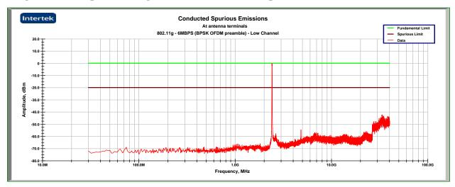
Lynx B1- 802.11g - 6MPS (BPSK OFDM preamble) - Low Channel
