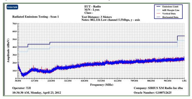
Lynx B - Peak Plot - 30MHz-1000MHz - 802.11b - 5.5Mbps - Low Channel
