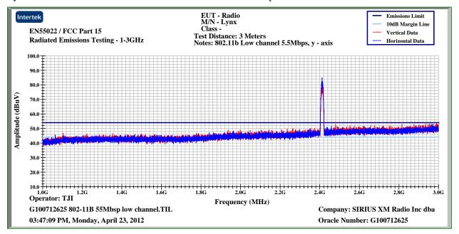
Lynx B - Peak Plot – 1000MHz-3000MHz – 802.11b – 5.5Mbps – Low Channel
