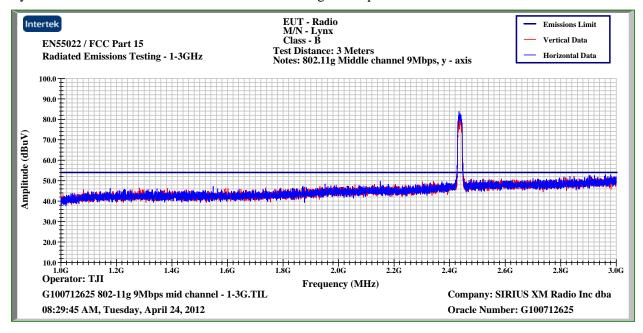
Lynx B - Peak Plot – 1000MHz-3000MHz – 802.11g – 9Mbps – Middle Channel
