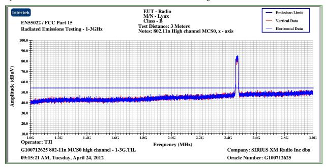
Lynx B - Peak Plot - 1000MHz-3000MHz - 802.11n - MCS0 - High Channel
