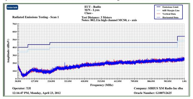
$Lynx\ B\ -\ Peak\ Plot-30MHz-1000MHz-802.11n-MCS0-High\ Channel$
