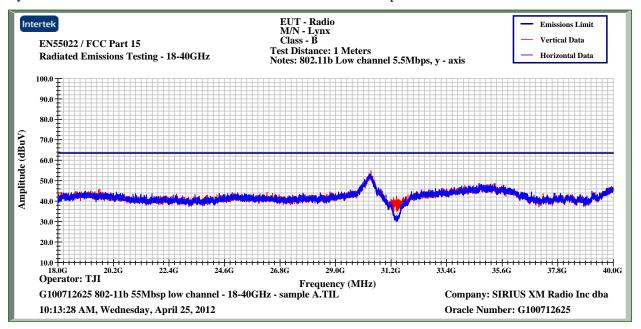
Lynx B - Peak Plot – 18000MHz-40000MHz – 802.11b – 5.5Mbps – Low Channel
