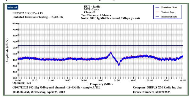
Lynx B - Peak Plot – 18000MHz-40000MHz – 802.11g – 9Mbps – Middle Channel
