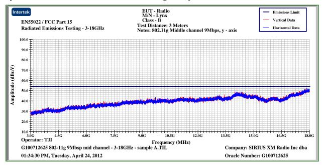
Lynx B - Peak Plot – 3000MHz-18000MHz – 802.11g – 9Mbps – Middle Channel
