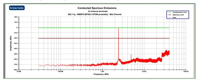
Lynx B1- 802.11g - 9MPS (BPSK OFDM preamble) - Middle Channel
