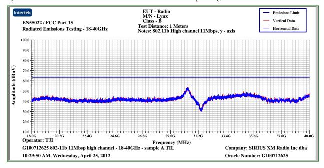
Lynx B - Peak Plot – 18000MHz-40000MHz – 802.11b – 11Mbps – High Channel
