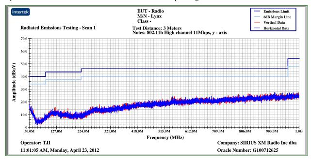
Lynx B - Peak Plot - 30MHz-1000MHz - 802.11b - 11Mbps - High Channel
