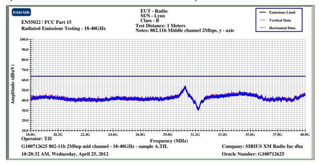
Lynx B - Peak Plot - 18000MHz-40000MHz - 802.11b - 2.0Mbps - Middle Channel
