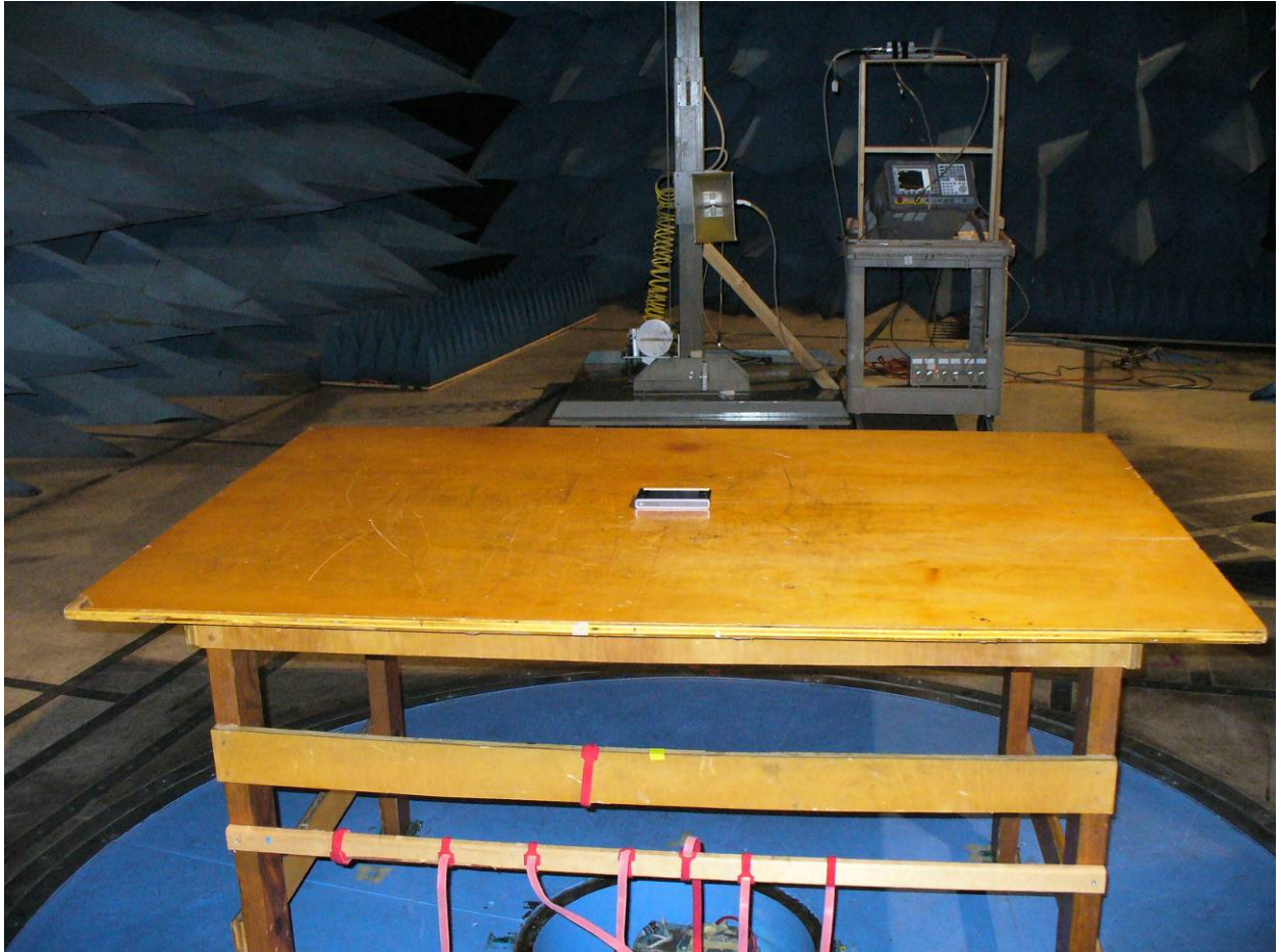
Figure 2: Radiated Emissions – X Position - Back View
