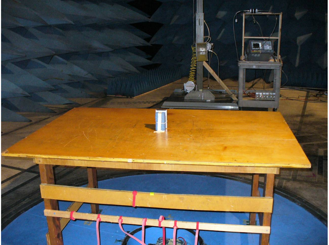
Figure 6: Radiated Emissions – Z Position - Back View
