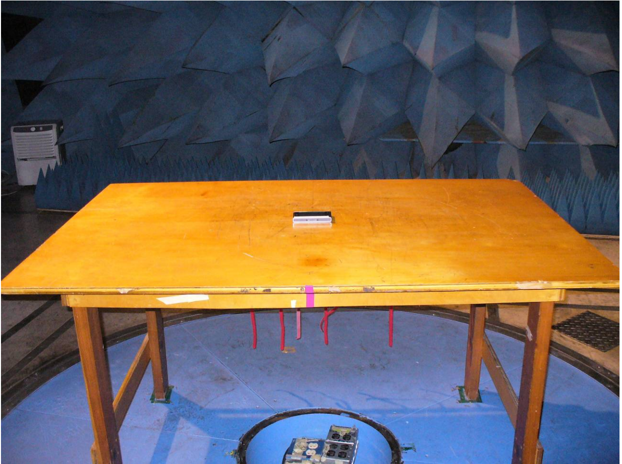
Figure 1: Radiated Emissions – X Position - Front View
