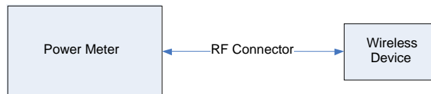
Figure 10-1 Power Measurement Setup
